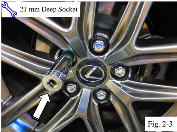
(c) Place the 21mm Deep Socket on top of the key. (Fig 2-3)
